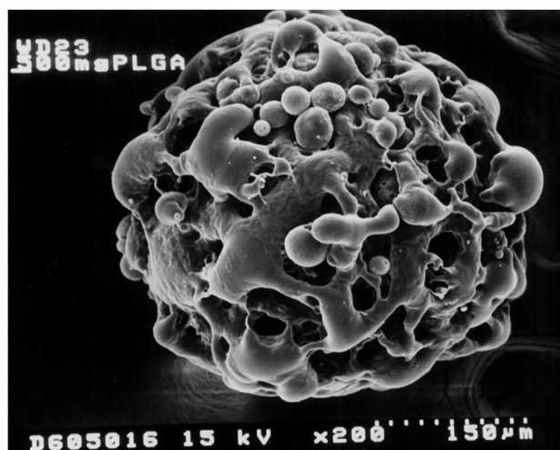
Fig. 1. Typical SEM photographs of microparticles prepared in presence of corn oil.
