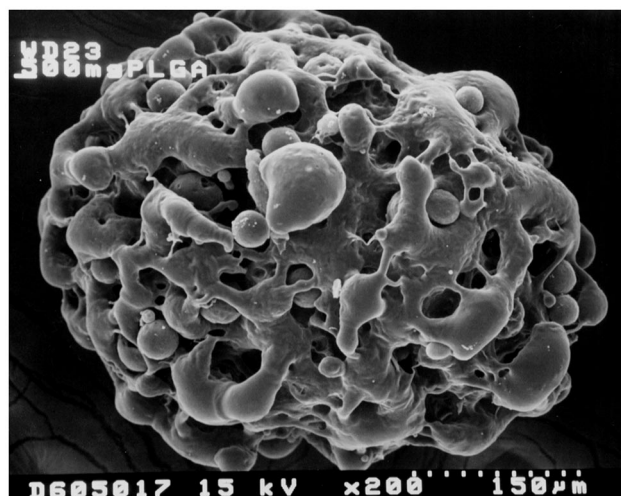
Fig. 2. Typical SEM photographs of microparticles prepared in presence of mineral oil.
